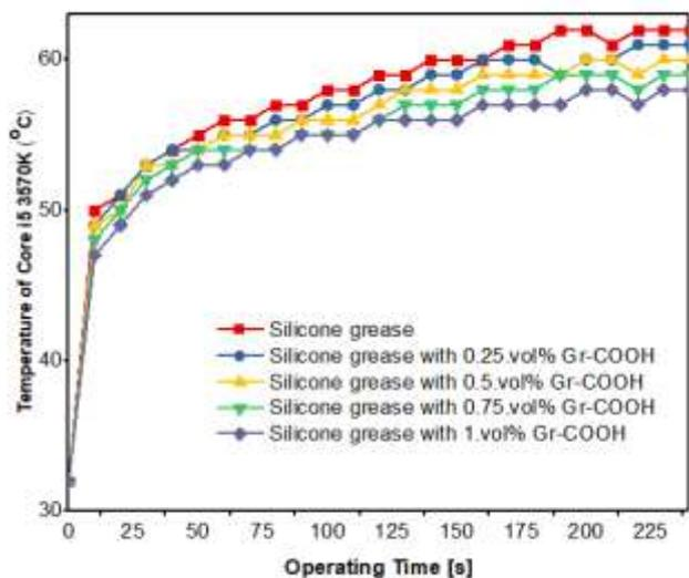
Fig.7. The measured temperature of the microprocessor as a function of the operation time in the case of using thermal grease
