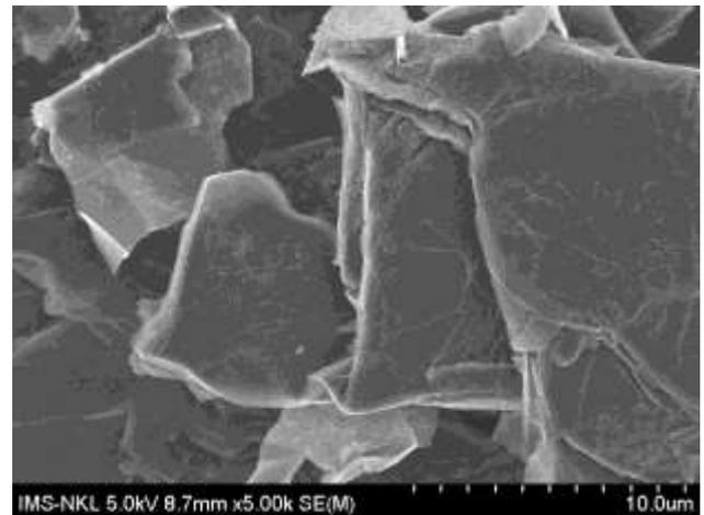
**Fig.3.** FESEM image of graphene nanoplatelets
